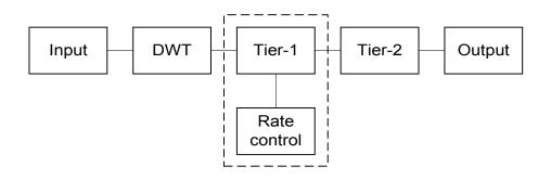
Fig.1 Image encoding process
